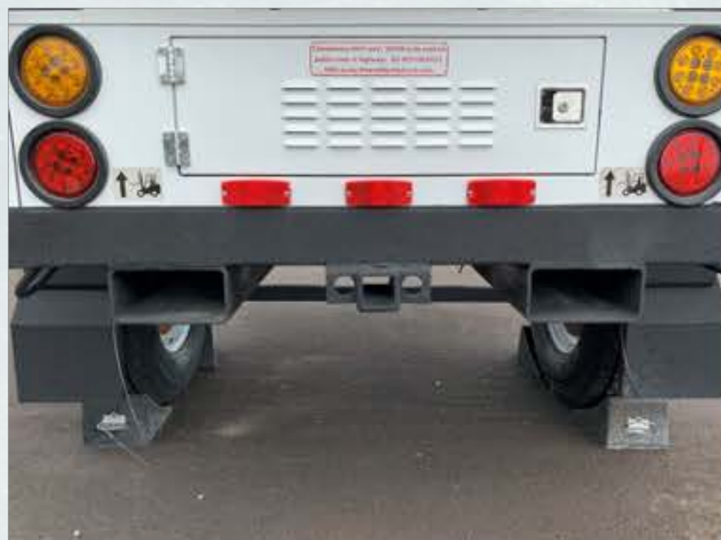
Steel Fork Pockets: Full length of trailer for easy loading, unloading, and added trailer strength
